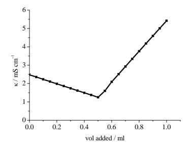
$\kappa$  decreases to the end point because mobile OH<sup>-</sup> ions are being replaced by less mobile Cl<sup>-</sup> ions. After the end point  $\kappa$  increases because of the addition of ions. The increase is rapid because of the high mobility of the H<sup>+</sup> ions.
