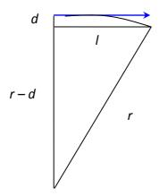
The distance to the screen is l and the displacement of the beam on the screen is d. By Pythagoras  $(r-d)^2+l^2=r^2$ , hence  $r=\frac{d^2+l^2}{2d}$
